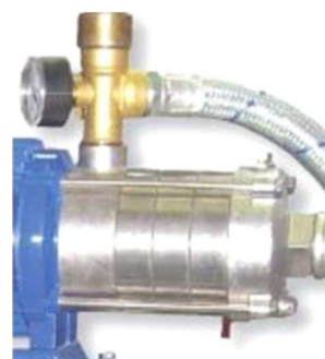
Fig 6: multistage pump outlet with manometer to replace with the transducer
